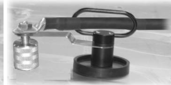
② Screw the earth to the metal sheet
